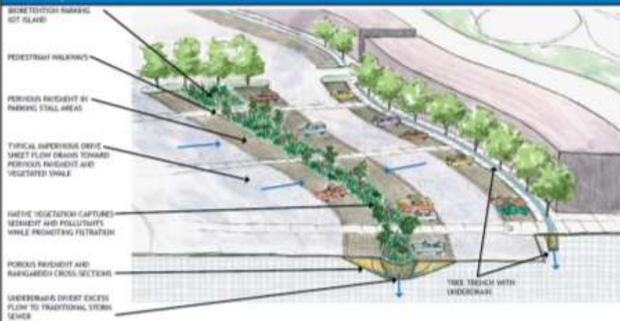
Figure 12.BIO.5 Bioretention Parking Lot Island (Source: Minnehaha Creek Watershed District)
